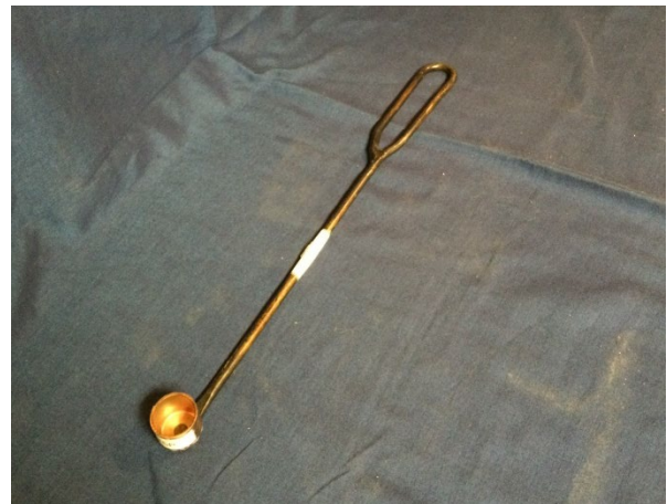
Figure 8. A long-handled bait dispenser can be constructed easily with a copper end cap, rivet, and ¼-inch rod. Compare the end-cap's capacity against a teaspoon cooking measurer to confirm correct volume.
