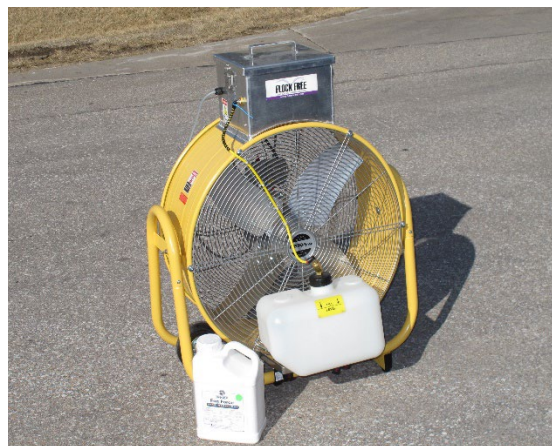
Figure 8. Fan used to disperse methyl anthranilate.
