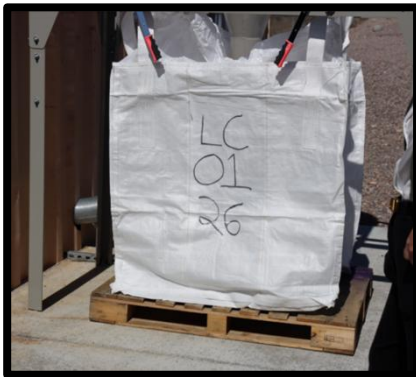
Super seed bag in which 1400 lbs. of the finely ground plastic from recycled pesticide containers is blown into.
