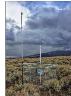
Station in sagebrush rangeland west of Dillon, MT with optional NDVI sensor pair measuring vegetation greenness, for tracking vegetation vigor and production.
