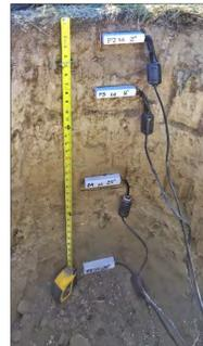
Soil pit near Roundup, MT. The probes record changes in soil water content, temperature, and soil water quality.
