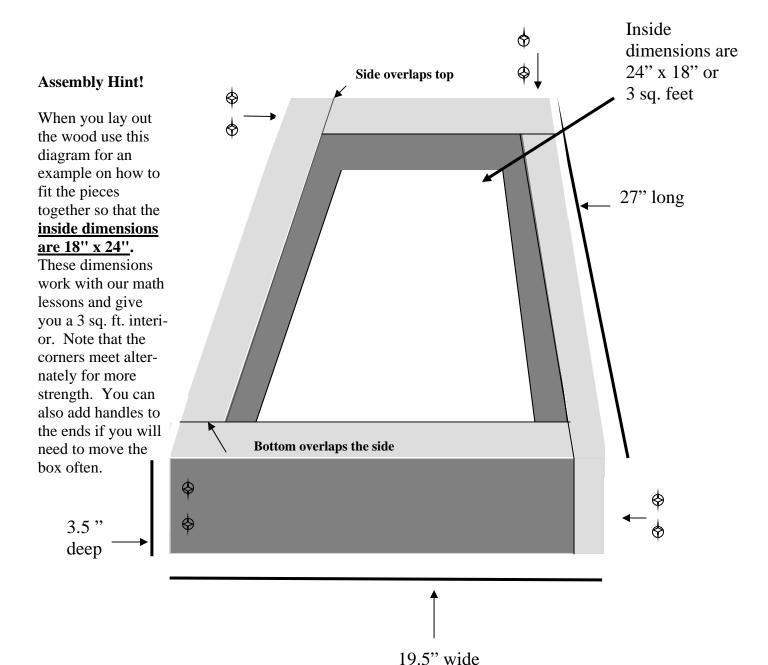
KEY: Fasten with screws at these joints, it is a good idea to predrill the holes.
