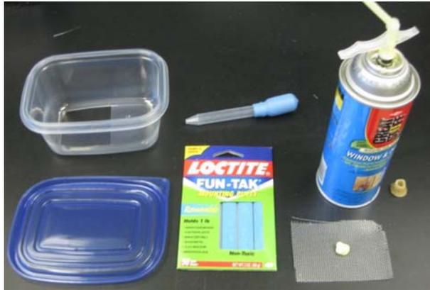
**Figure 3. Items needed to make a starter box**
